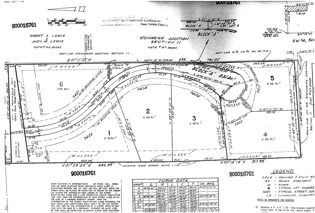
D Denotes a 4" x 4" x 36' long precast concre! cross cast in top to be set, where shown, fl 1, the undersigned, hereby certify that to the best of my professional knowledge and belief the within plat accurately represents a survey performed under my supervision during the month of June. 1989 of the following described real estate:
