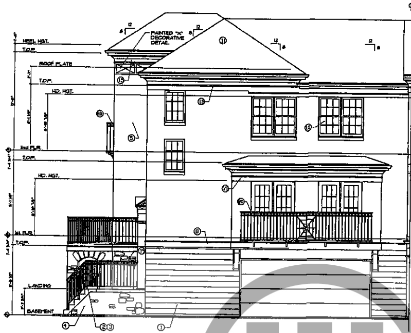
UNIT 'D2' BUILDING 9 - SIDE (NORTH) ELEVATION 1/4" = 1'-0"
